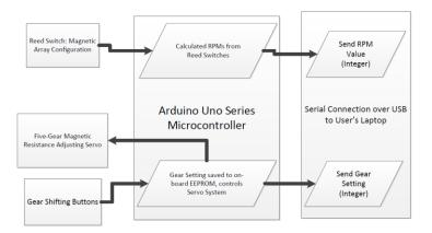
Figure B-1: The Block Level View
