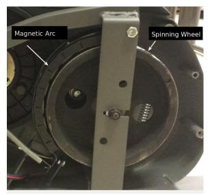
Figure D-3: Magnetic Arc and Spinning Metal wheel
