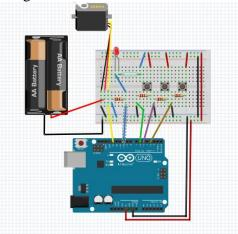
Figure B-8A: The Fritzing Diagram showing the Arduino Connections. Two of the buttons represent the Reed Switches, the third represents a reset state.
